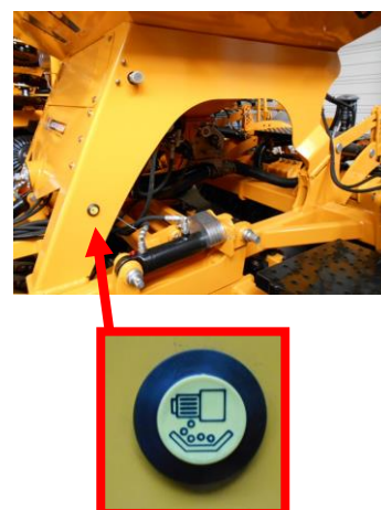
Figure 17: button to activate the seeding rate test
