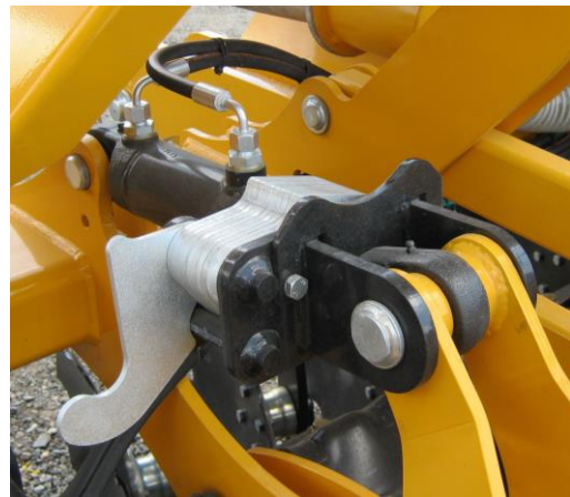
Figure 19: Shims on the cylinder
