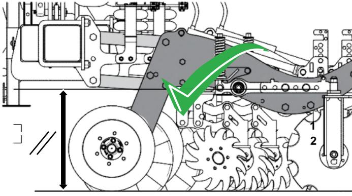
Set the implement down on the ground and adjust the pressure in the air cushions serving to set the working depth of the parallelogram. Ensure that the arms of the parallelogram are virtually parallel to the ground. Move forward a few meters to drive the implement into the ground, then adjust the vertical alignment with the top link of the tractor.
