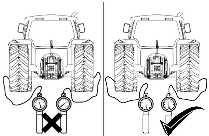
Check the general condition and the pressure of the tractor tires (refer to the tractor operator's manual). The pressure must be identical on both sides of the tractor to ensure that the implement is level.
