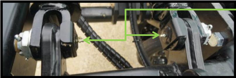
Cylinders pivot point grease-zerks
