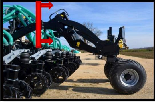
For transport the lift assist system is disconnected at the red line.
