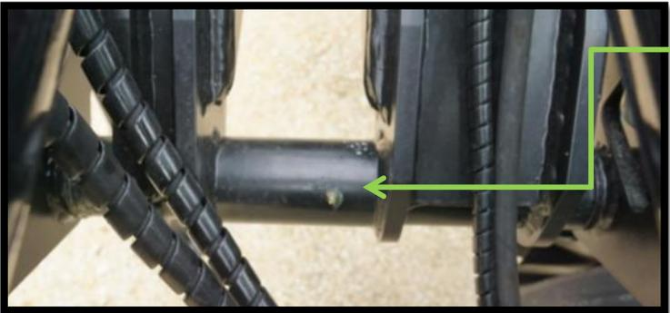
Wing pivot point grease-zerk
