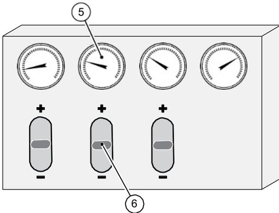
Where ground conditions are good (dried soil), the pressure in the press roller system can be increased.
