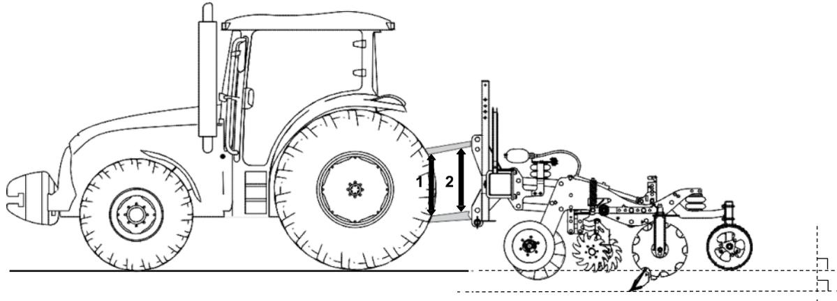
The top link must be attached to a hole in the coupling yoke. It must always be placed at a higher level on the implement side than the tractor side. When working, once the implement is in the ground, set the lifting control to floating.
