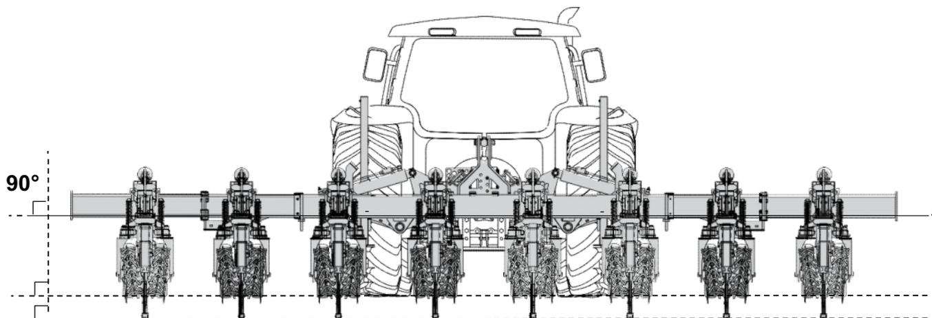
In the working position, the frame of the implement must be level from left to right. This normally occurs when:
