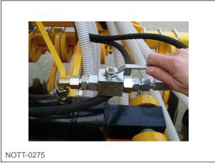
5 - Actuate the tractor's folding hydraulic control valve up to the mechanical stop point.
