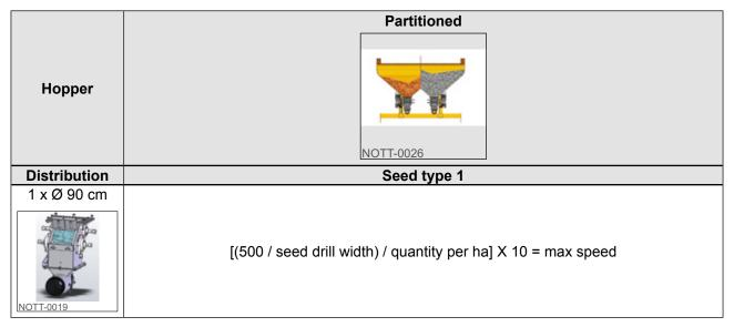
For sowing two seed types and/or fertilisers with a 2 x Ø 70 cm distribution unit:
