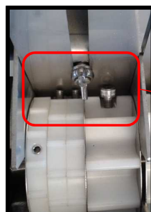
1 small spline engaged
