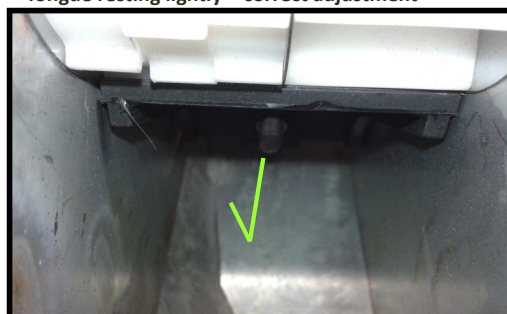
Tongue resting lightly = correct adjustment
