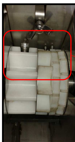
2 small splines engaged
