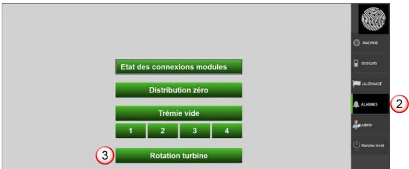
3. Press the button corresponding to an alarm to activate it (it will appear in green) or deactivate it (it will appear in grey).
