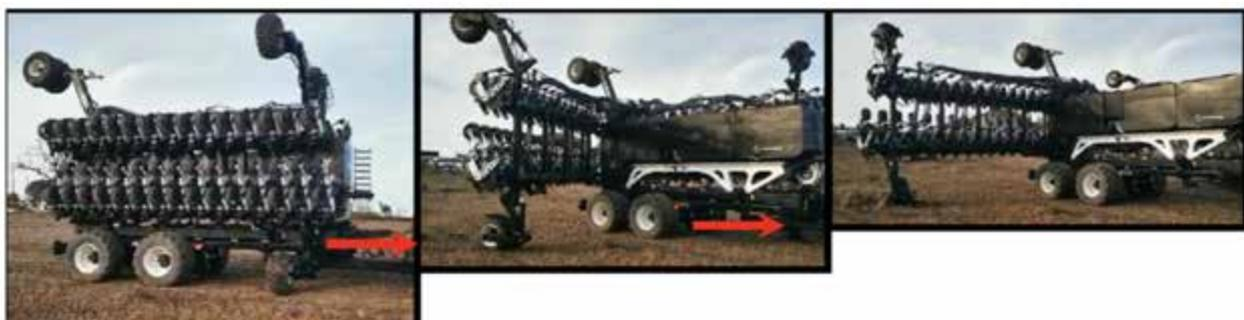
8. Activate the frame cylinders on the tractor to lower the frame completely.
