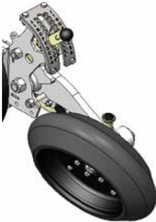
Pull the lever out and position it on the desired notch using the graduated adjustment plate.
