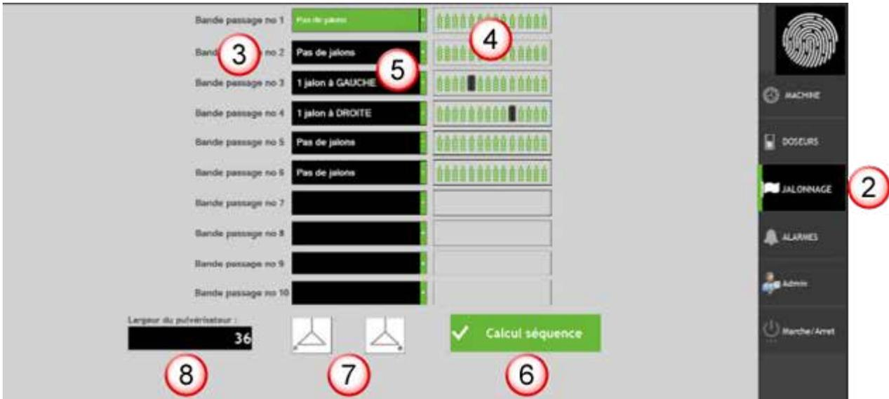
3. Press button (6) **Sequence calculation** to configure the tramlining.
