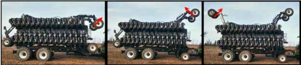
4. Lift button 4 to unfold the side gauges.
