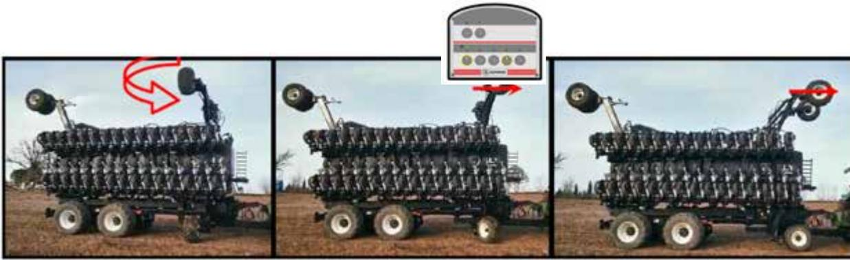
9. Lift button 2 to fold the lift assist and the side gauge wheels.
