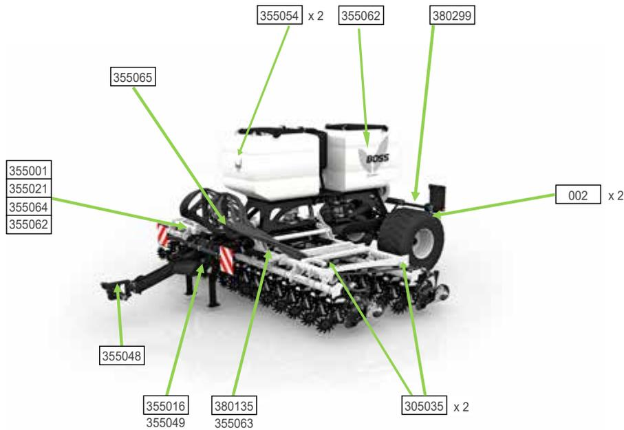
The safety stickers with the supplement 'x 2' are located on both sides of the machine.
