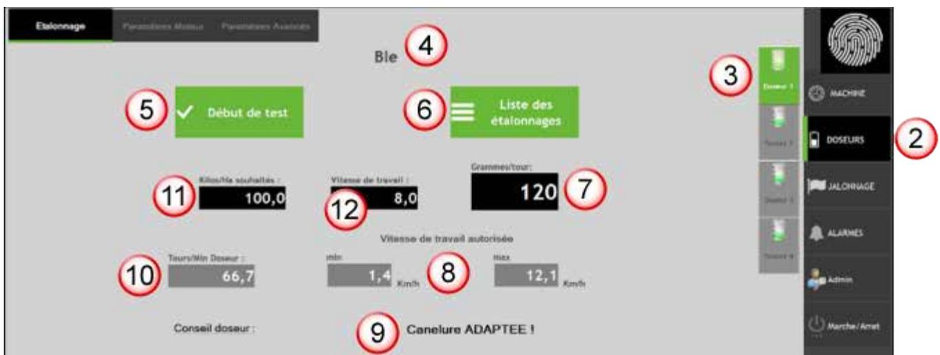
3. Select the dispenser to be configured by pressing the corresponding **Metering unit X** button (3).
