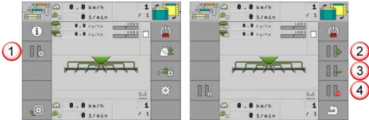
2. Press button (2) **Additional manual run** to manually force an additional run.
