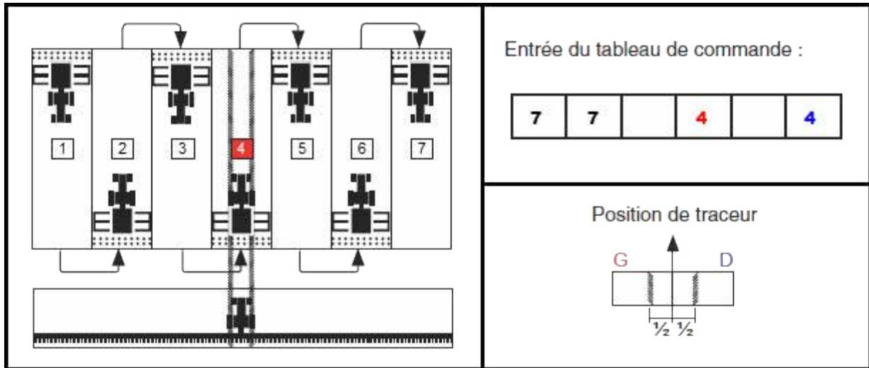
1. In the table, select the row 7 : 7 \_ 4 \_ 4 with the control wheel and then press the control wheel to confirm.
