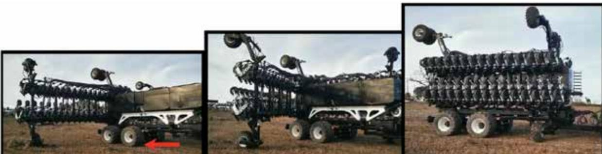
7. Activate the frame cylinders on the tractor to complete the lifting of the frame and to be able to lock the wings at the end of the folding process.
