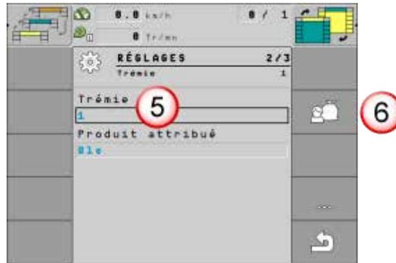
6. Press field (5) **Hopper** to select the hopper in which the seed is located.
