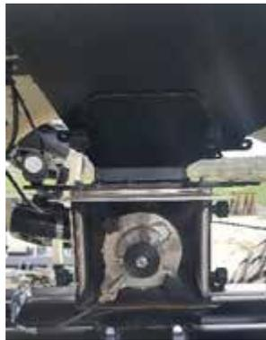
4. If necessary, set the metering unit to forced operation to completely empty the bottom of the hopper.
