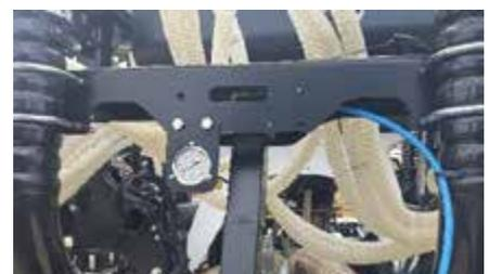
To change the pressure, turn the adjustment wheel clockwise with an Allen key to increase the pressure and anti-clockwise to decrease it.
