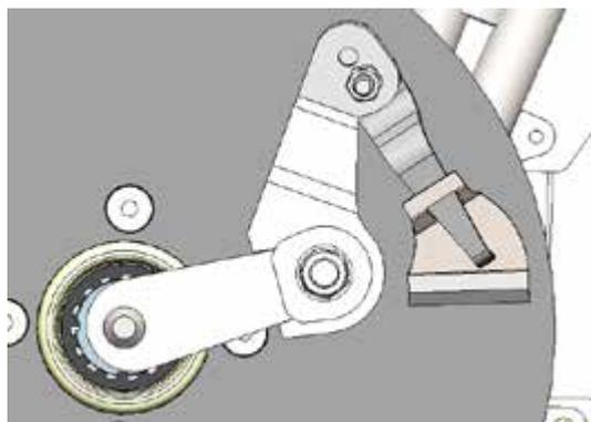
1 : The entire length of the scraper blade should be in contact with the disc and 10 - 12 mm from the outer edge of the disc to avoid damage to the skimmer.
