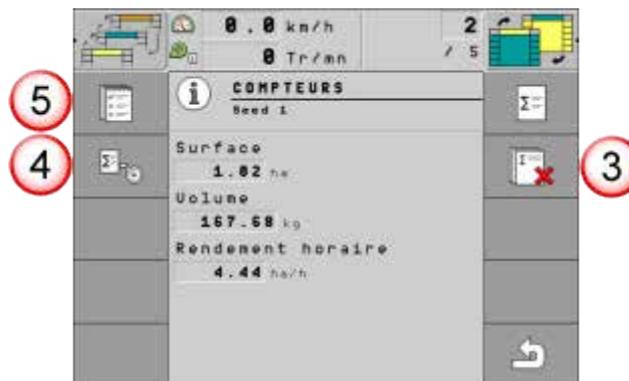
3. Press button (3) **Reset** to reset the counters to zero.
