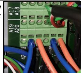
6 - The hopper sensors are connected to S1 and S2
